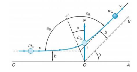
$\alpha$  particle trajectory is hyperbolic Scattering angle is related to impact par.
