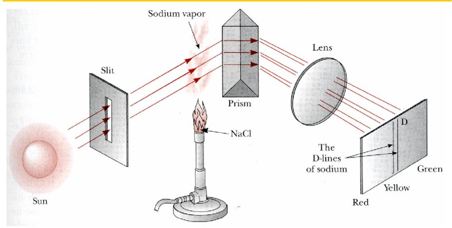
D lines darken noticeably when Sodium vapor introduced Between slit and prism
